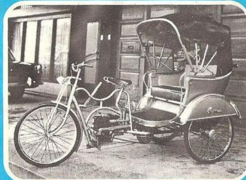
Model - V9M Passenger Pedicab with gasoline engine. Weight ..... 155Kgs. 107" X 45" X 67"
