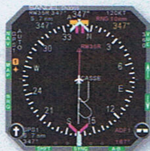
The Sandel EHSI depicts final approach to RW 35R at Denver's Centennial Airport. The active leg is shown in magenta and the other legs are in white.
