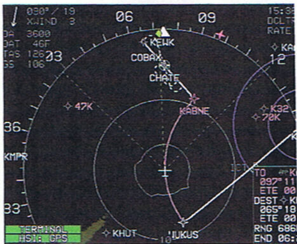
The moving map, shown above, depicts the aircraft halfway through the DME arc. The final approach segment turns away from the VOR. The missed approach is shown as a dotted white line returning to hold at the CHATE intersection. The light blue ring around the aircraft symbol is the "dead stick" glide area.
