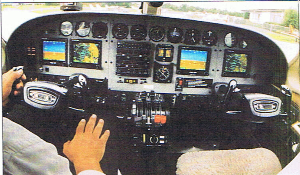
The FlightLogic EFIS, shown here in Chelton's Cessna 421, features four liquid crystal displays. At the far left is the primary flight display. The remaining three multi-function displays can be set up to show terrain, waypoints and other information.
