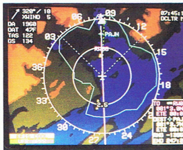
The TAWS display shows an approach into Juneau, Alaska. Black is used for terrain more than 2,000 feet below the aircraft, dark olive for terrain between 500 and 2,000 feet down, and light brown for terrain at or above the aircraft's altitude. Amber and red, not used here, show hazardous terrain ahead. The dead stick glide area is outlined in light blue.
