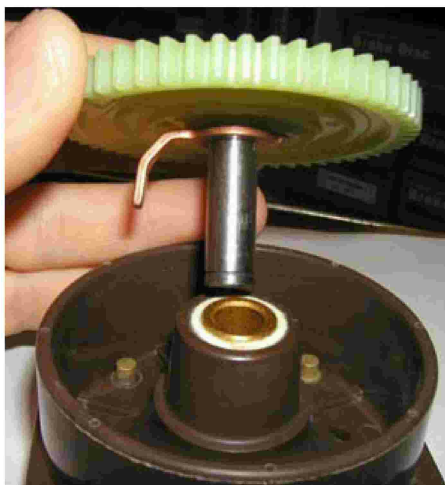
A 500-hour disassembly inspection of the TCM S-20 magneto is important and prudent, but it's not required by regulation.
